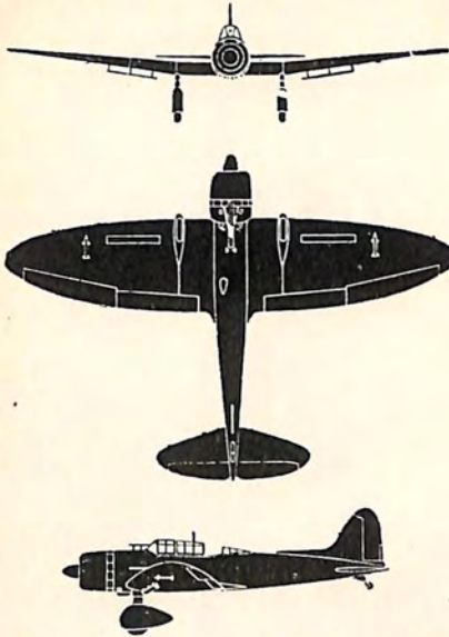
TYPE 99 DB VAL Mk2 Span 47' 7" Length 35' 5"
